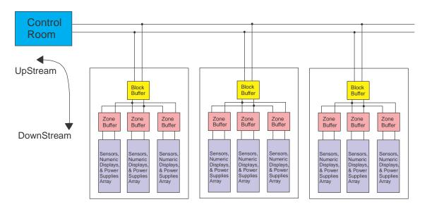
For the proposed site of 1200 sensors, across three levels we estimate the use of 3 ZoneBuffers and 1 BlockBuffers per level. A total of 12 data buffering devices.
